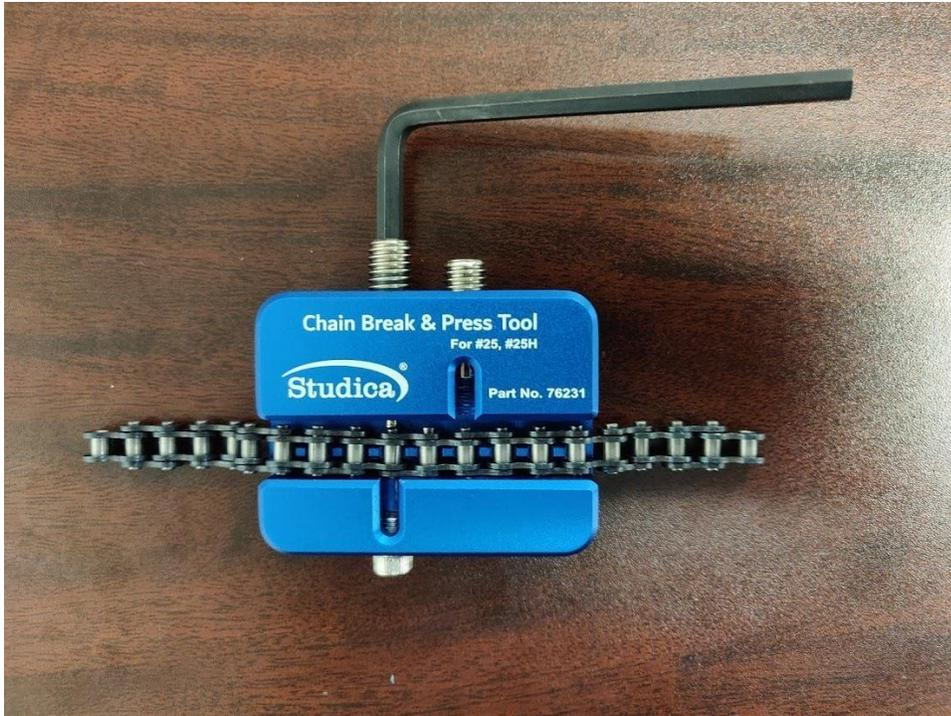
Start to screw in mandrel to remove pin.
