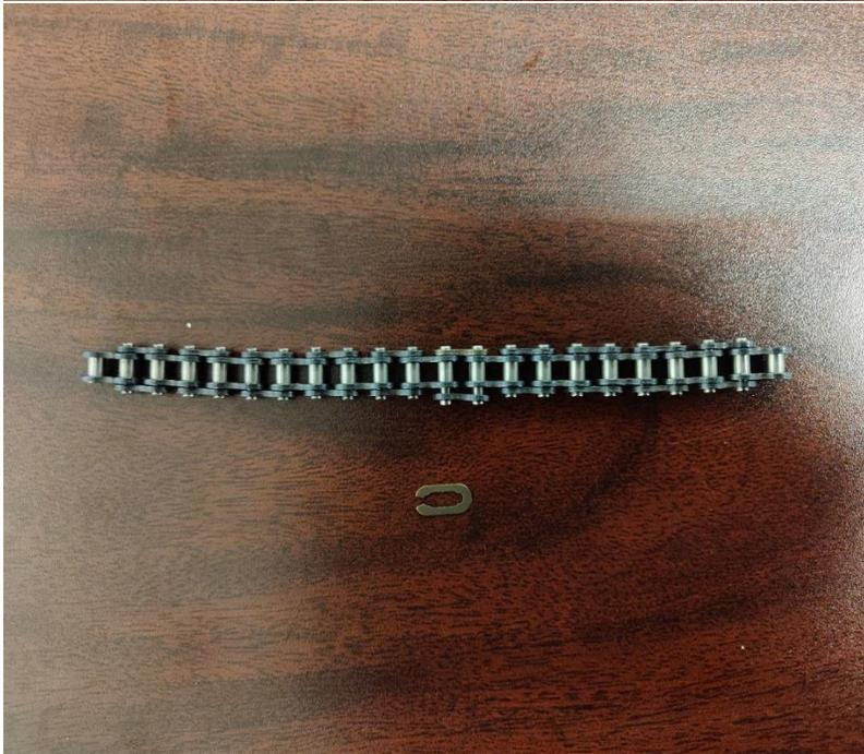
Push plate into bottom of both pins.
