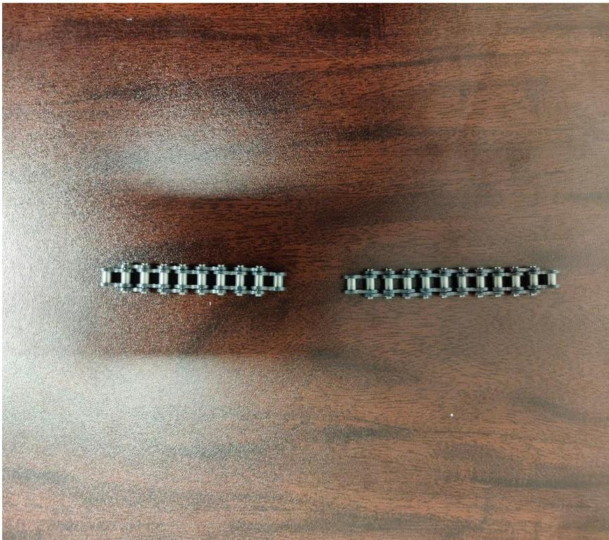
Although not provided with the Chain Breaker Tool, chains will come with master links to attach two chains that have 2 male connections, as opposed to 1 female and one male (pictured above).
