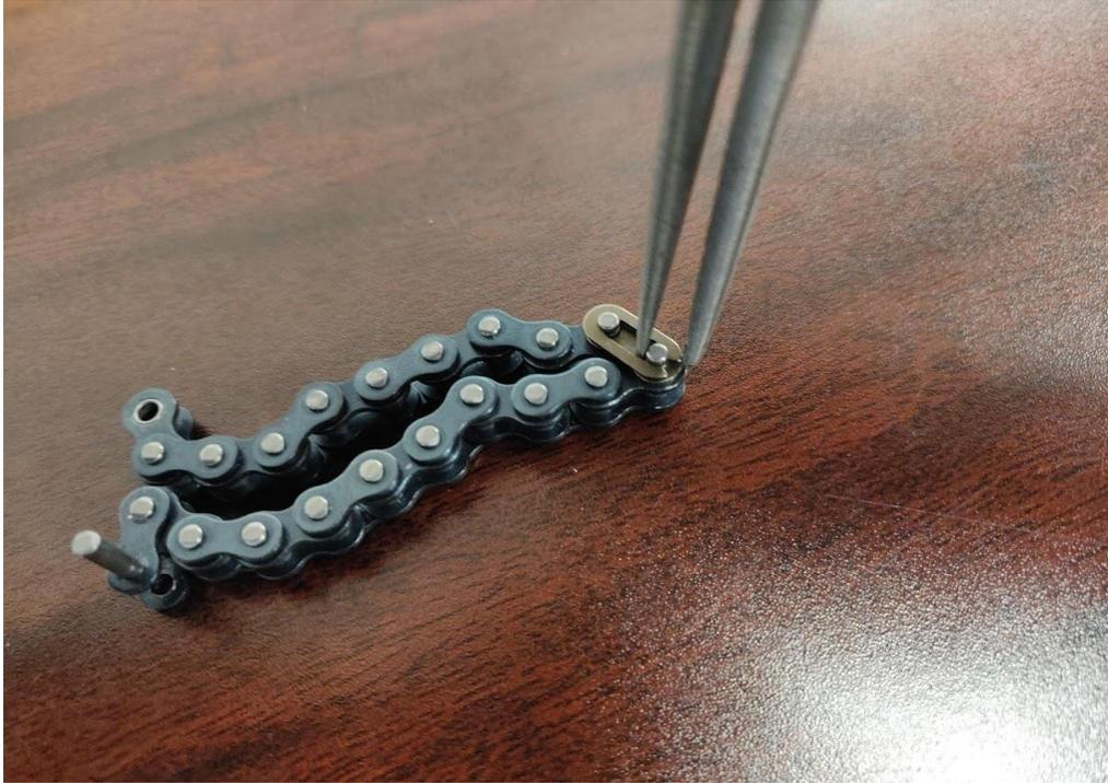
Place pliers at open side of master link. Press pliers together with pin and master link as pictured above.
