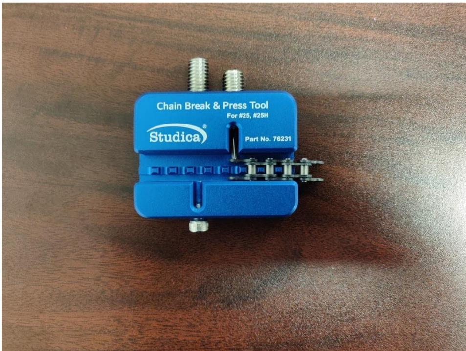
Put chain with pin attached to top link under the cup point.
