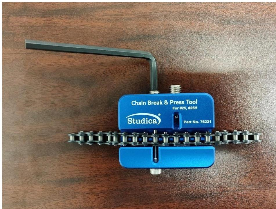
Keep screwing until pin can no longer be pushed.
