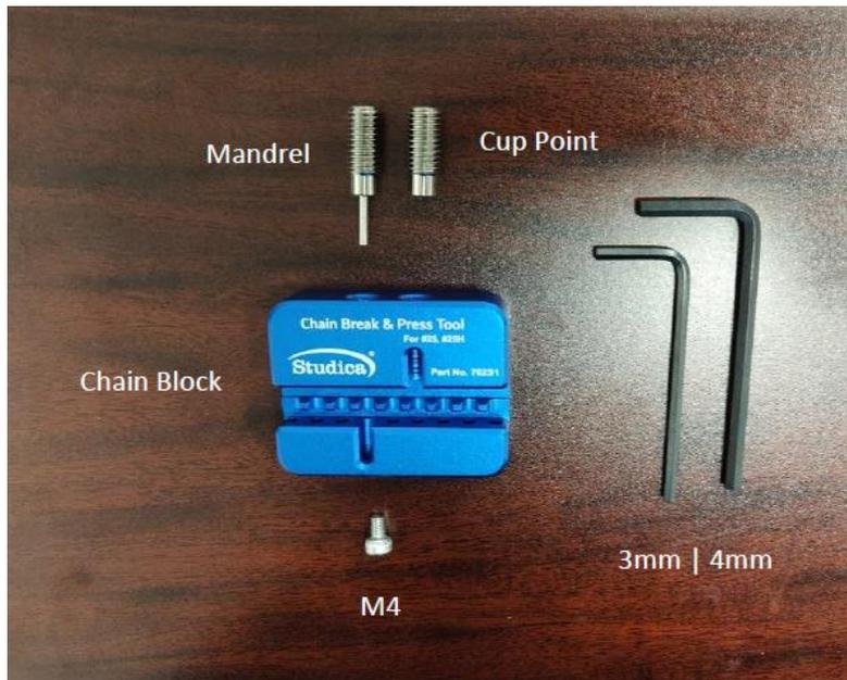
Pictured above are all the parts that come with the Chain Breaker Tool.
