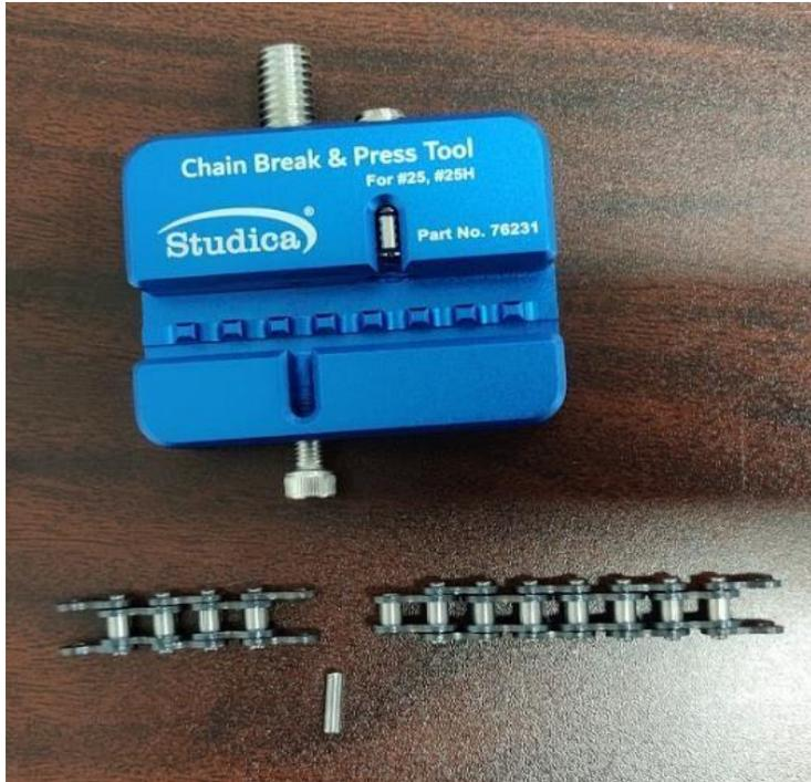
Remove chain(s) and pin from chain block.
