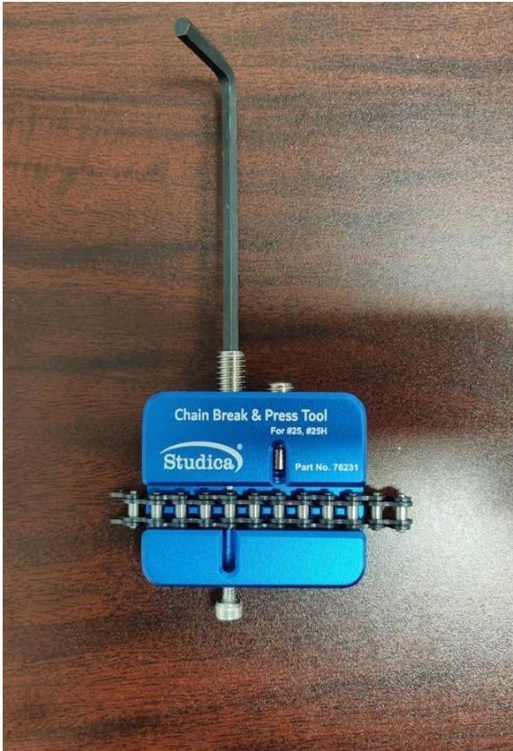
Add chain as pictured above, with the area you want to break under the mandrel. Start turning the mandrel clockwise so the mandrel screws in, until the pin has been pushed out.
