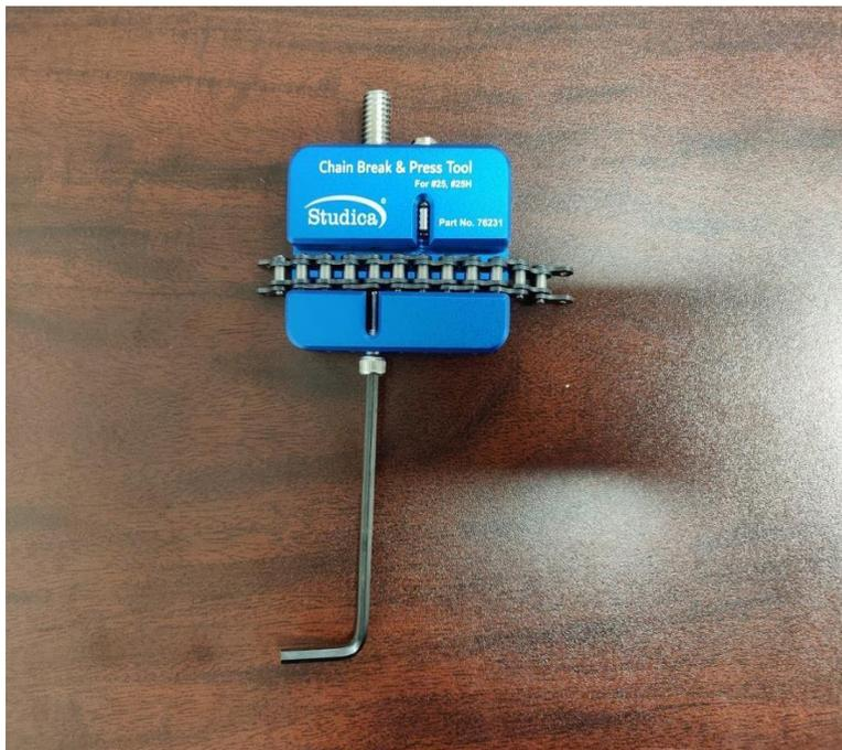
Start screwing with the 3mm Allen key until the pin is attached to part of a chain.
