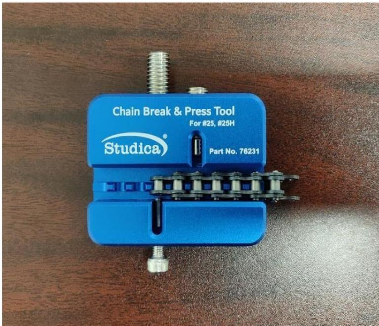
Put pin as shown above and insert first chain.
