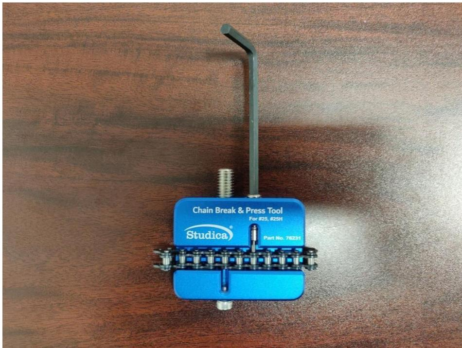
Screw in the cup point using the 4mm Allen key until the cup point touches the chain.
